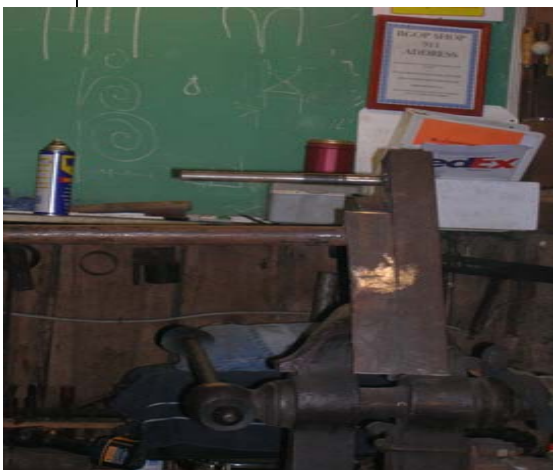
Dick Smith's coil spring straightening jig which incorporates a fulcrum and a straightening lead
