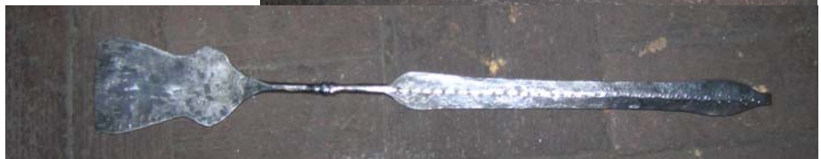
3 spatulas by Bill Wojcik. The larger was forged from 9" of 1-1/2"x 3/8" the smaller two from 9" of 1"x5/16" stock
