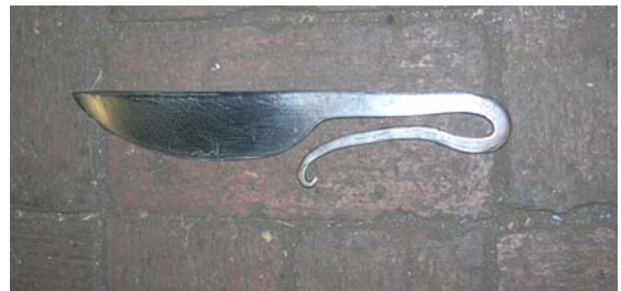
This is one of the two knives Wade Adkins brought, one was from a leaf spring, and one from a lawnmower blade.
