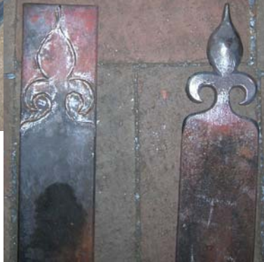
Fleur de Lis made by Phil Heath and the chisels he made to create them. Notice the chisels are each for a specific side
